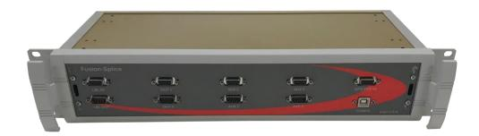
The system reads in strings in real time (invisible to the parent system), cuts, pastes and processes specific fields and then generates required strings that are output to third party instruments.
