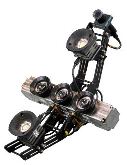
features. These descriptor vectors are then used to match features between the three cameras. Once the features are matched between cameras, known camera intrinsics (focal length, distortion, and optical center) and extrinsics (camera location and orientation) are used to triangulate the features, generating a sparse point cloud in the left camera frame. The 2D and 3D points, along with feature descriptors are then passed into the navigation engine.
